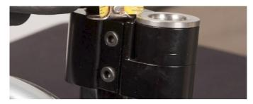
Place one Wheelchair Clamp at about the midpoint of the wheelchair cane. Lightly tighten the Clamp screws using the 4mm hex key.
